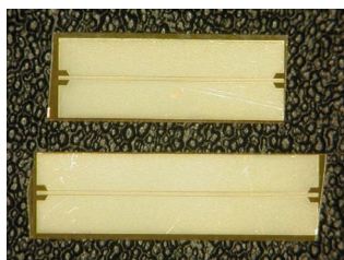
Fig. 4. Realized flexible coplanar waveguide test samples
